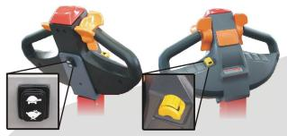
Roller to control the descending speed of the Forks
